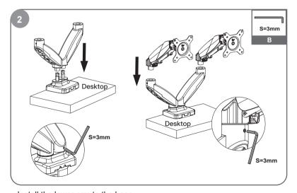
Install the lower arm to the base. Insert the gas spring arm above the lower arm.
