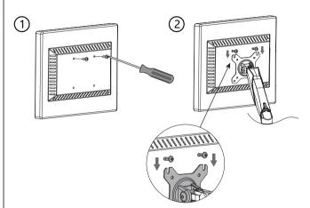
3 Flush surface installation: Install the lower two screws and fasten the upper two screws.
